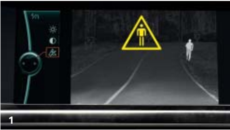
1. BMW Night Vision recognizes people and displays their position and distance from the car, sounding a warning if they are too close. 2. The controls for the intercom and alarm systems are within easy reach of the driver's hand, yet hardly noticeable to observers outside the vehicle. 3. Functional bookmarks allow security-related functions to be activated at the touch of a button. 4. Official-use equipment is among the systems that can be controlled via iDrive.
