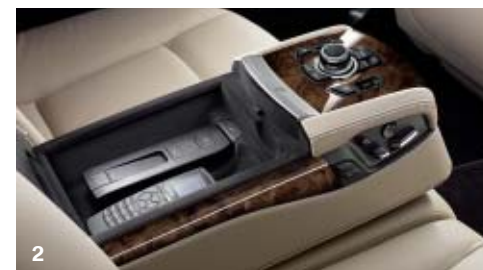
1. iDrive controller in the rear centre console for operating entertainment, telephone and air conditioning systems (optional). 2. Preparation for mobile phone/separate telephone in rear (optional). 3. Cool box in centre console.
