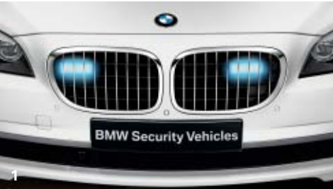
1. LED flashing lights can be located discreetly behind the BMW kidney grille. 2. Flag holder for diplomatic and official use. 3. Flashing lights for the roof can be attached to a mounting bar easily and quickly. 4. A radio or firearm bracket can be mounted in the centre armrest.
