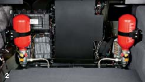
1. Emergency exit via front windscreen, with pyrotechnic detonation. 2. Fire extinguisher system with extinguisher reservoir in luggage compartment. 3. Emergency fresh-air system with air reservoir in luggage compartment.
